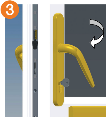
3 Push the handle down to retract the hook bolts and the latch. This allows the door to be opened.
